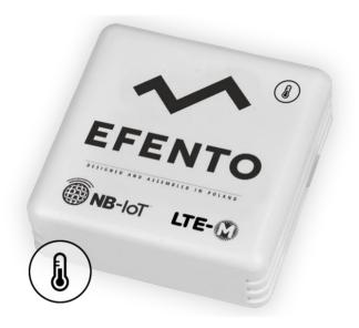
NB-IoT / LTE-M temperature sensors are used for remote temperature monitoring, in places where constant supervision is required, such as medical refrigerators, pharmaceutical wholesalers, museums, archives – especially suitable for monitoring distributed objects (transformer stations, pumping stations).
