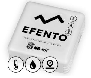
Wireless temperature, humidity and atmospheric pressure loggers are used for indoor measurements, among others in warehouses, hospitals, museums or airports.
