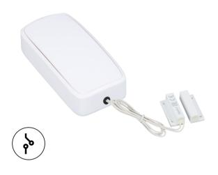
Wireless open / close sensor detects and logs in its memory events of door opening and closing. If a change of state is detected, the device immediately sends the notification to Efento Cloud or other IoT cloud platform. The device uses magnetic sensor to detect open / close event.
