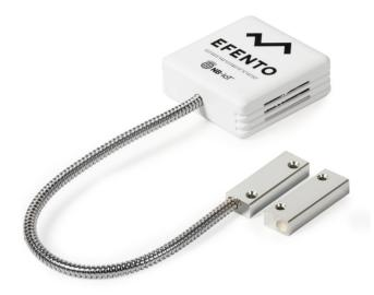
Wireless open / close sensor detects and logs in its memory events of door opening and closing. If a change of state is detected, the device immediately sends the notification to Efento Cloud or other IoT cloud platform. The device uses magnetic sensor to detect open / close event.
