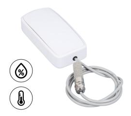
The sensor is equipped with an external, temperature and humidity probe with a length of 1m, allowing measurements in places where the sensor cannot be placed directly.
