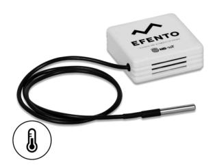
The logger is equipped with an external, waterproof probe which allows to measure the temperature in points there where the sensor cannot be placed directly. The probe is available in two variants: standard or intended for contact with food, in the form of a sharpened skewer.
