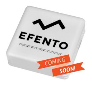
Efento LTE-M / NB-IoT wireless carbon monoxide (CO) logger measures gas concentration and transmit its values over a cellular network (Narrowband IoT or LTE-M). On top of the gas concentration, the logger also measures temperature and humidity. Sensors are also equipped with Bluetooth Low Energy interface, which allows quick and easy configuration with a smartphone. Efento LTE -M / NB-IoT gas sensors can be integrated with any cloud platform.
