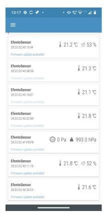
Remove protective tape from the logger's battery holder. Open the application, after a few seconds the application will automatically detect all sensors within range of your phone / tablet. The list shows the names of the sensors, their serial numbers and their current measurement values.
