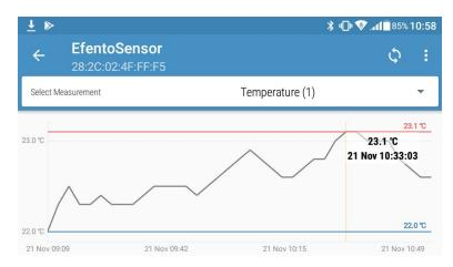
Click on the chart in the general view to zoom it in. Use your fingers to zoom in / out the chart and scroll it. Red and blue lines on the chart indicate the minimum and maximum values in the measurement series. If the sensor measures more than one physical value, select the one you want to display on the chart using the dropdown at the top of the screen.
