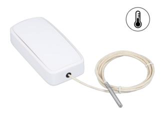
Efento wireless high temperature NB-IoT sensors are designed to monitor the operation of devices requiring constant high temperatures, e.g. bakery ovens, industrial drying ovens. The loggers are equipped with a 1m probe with a Pt1000 sensor, which can be safely placed in a place with high temperature.
