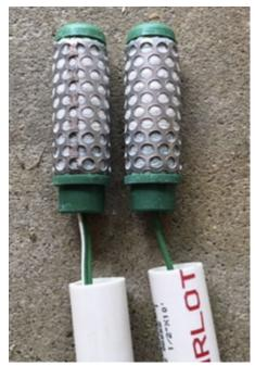
The probes should be placed at the bottom of the hole, so that the soil moisture probe has direct contact with the soil.
