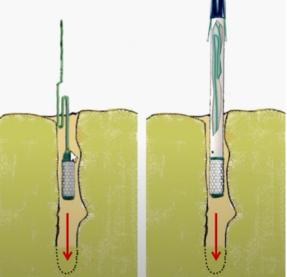
The rest of the mixed mud should be used to fill the spaces in the hole once the probes have been placed.
