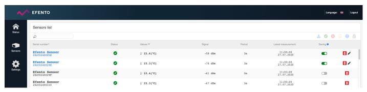
You can manually select which sensors should synchronise the data with Efento Cloud
