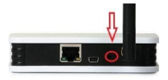
Quickly press the button twice to switch Efento Gateway to configuration mode
