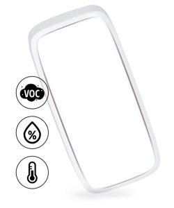
Wireless temperature, humidity and air quality logger is designed to monitor indoor climate conditions. The device measures air quality based on the concentration of volatile organic compounds (VOC) and calculates IAQ (Indoor Air Quality) representing air quality in the room based on the Bosch patented algorithm. Volatile organic compounds are substances derived from many indoor products, including from paints, cleaning agents, solvents, alcohol or glue.
