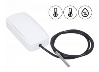
The logger is equipped with internal temperature & humidity sensor and external temperature probe (waterproof) which allows to measure the temperature in points there where the sensor cannot be placed directly. The probe is available in a few variants: standard, flat, screw or intended for contact with food.
