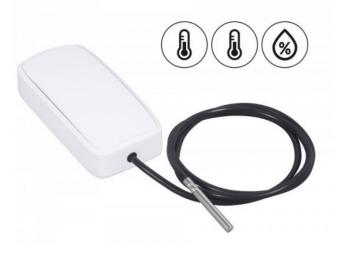
The logger is equipped with internal temperature&humidity sensor and external temperature probe (waterproof) which allows to measure the temperature in points there where the sensor cannot be placed directly. The probe is available in a few variants: standard, flat, screw or intended for contact with food.
