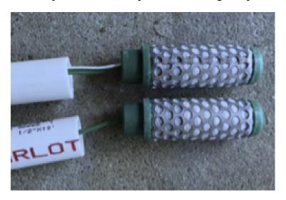
Dig a hole for the soil moisture sensor and mix a dug soil with water to the consistency of honey. The bottom of the dug hole should be poured with prepared slurry. The probe should be placed at the bottom of the hole, so that the soil moisture probe has direct contact with the soil. The rest of the mixed mud should be used to fill the spaces in the hole once the probes have been placed
