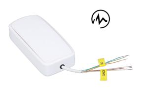
Efento 4-20 mA sensor interface allows users to connect any type of analog sensor. Device can be equipped with up to two analog interfaces (2 x 4-20 mA). Sensors can be powered either from the device's battery or by an external power source. Data from the analog sensors can be presented as current (4-20 mA) or converted to other measurement types once it reaches the Efento Cloud platform.
