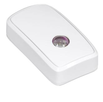
Efento NB-IoT loggers transmit the data over cellular network (Narrowband IoT) and do not require any additional devices (router, gateway, etc.). Sensors are also equipped with Bluetooth Low Energy interface, which allows quick and easy configuration with a smartphone. Efento NB-IoT sensors can be integrated with any cloud platform. You can use a free mobile application to configure the device and read the data from its memory.
