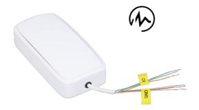
Efento 4-20 mA sensor interface allows users to connect any type of analog sensor. Device can be equipped with up to two analog interfaces (2 x 4-20 mA). Sensors can be powered either from the device's battery or by an external power source. Data from the analog sensors can be presented as current (4-20 mA) or converted to other measurement types once it reaches the Efento Cloud platform.
