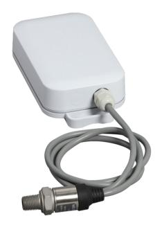
Pipe pressure sensors can be used to monitor the pressure of liquids or gases in the pipes. They are ideal for monitoring and preventing leakages from water pipes or any other pipe-based systems. The second popular use case of pressure sensor is monitoring of tank level based on the liquid's pressure.
