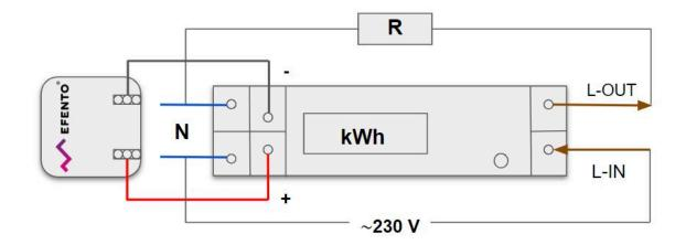
Efento electricity pulse counter - wiring scheme
