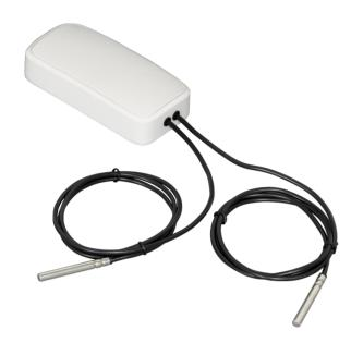
The logger is equipped with two an external, waterproof probe which allows to measure the temperature in points there where the sensor cannot be placed directly. The probes are available in two variants: standard or intended for contact with food, in the form of a sharpened skewer.
