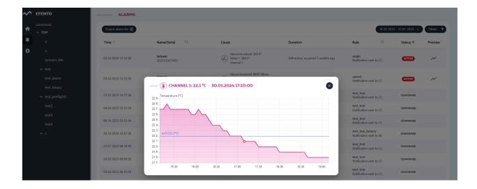
It is also possible to preview the sensor's measurements from the period of the alarm occurrence. After pressing the serial number of a device on the alarm list, the user will be redirected to a page presenting detailed data about the device and its complete measurements over a 4-hour period, including the moment of the alarm occurrence, marked with a red circle on the chart.
