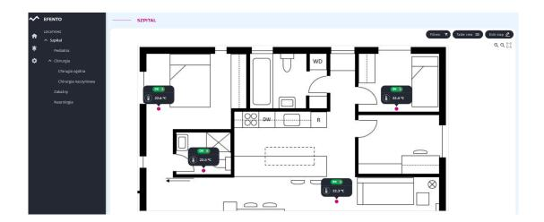
You can customize the display of sensor information. By clicking the *Edit* button, select which details should be shown: name, serial number, status, and current measurements. If all fields are unchecked, sensors will appear as colored dots, with the color indicating their status: green for ok, red for alarm, yellow for low battery, and gray for lost.
