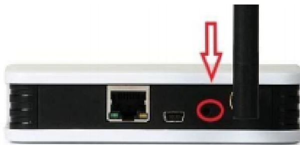
*Quickly press the button twice to switch Efento Gateway to configuration mode*
